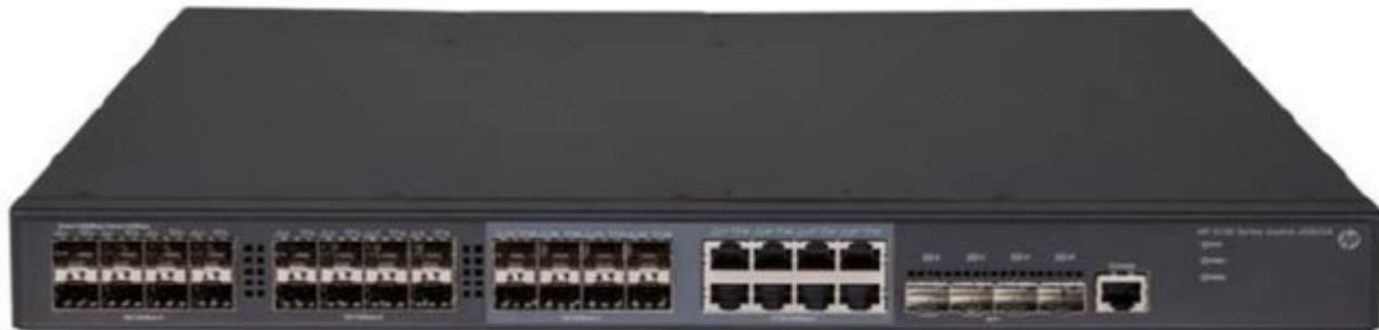
**HPE FlexNetwork 5130 24G SFP 4SFP+ EI Switch (JG933A)**
